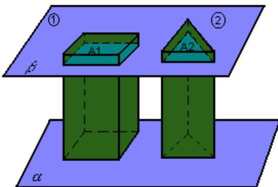
$$\text{all } \beta \text{ e } A_1 = A_2 \Rightarrow V_1 = V_2$$
